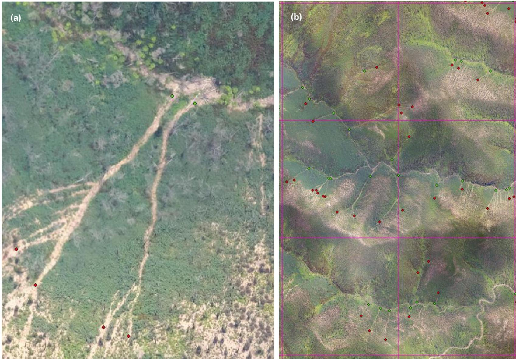
**Figure 2:** (a) and (b) show mapping of debris flow (depositional) fans (as green dots) and channel initiation points (as red dots) (figure (b) includes a 1km<sup>2</sup> grid)
