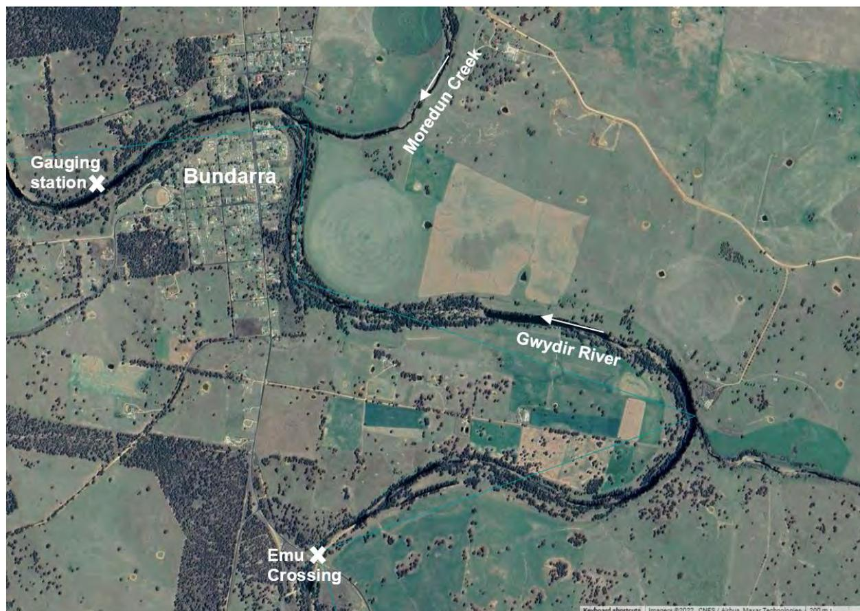
**Figure 4: Location of Emu Crossing on the Gwydir River showing how Moredun Creek is downstream of the crossing, which is the Plan's cease to pump reference point, rather than the gauging station downstream of Bundarra**
