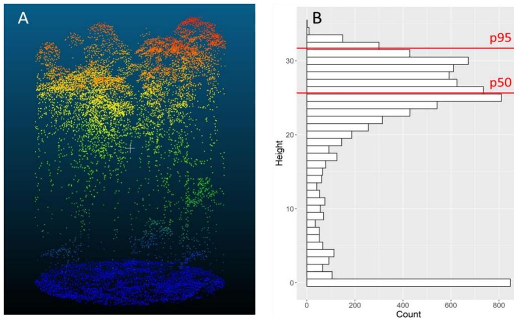
**Figure 7. Example of a lidar point cloud over a plot (A) and the resulting distribution of height values (B), with the 50<sup>th</sup> and 95<sup>th</sup> percentiles shown in red.**
