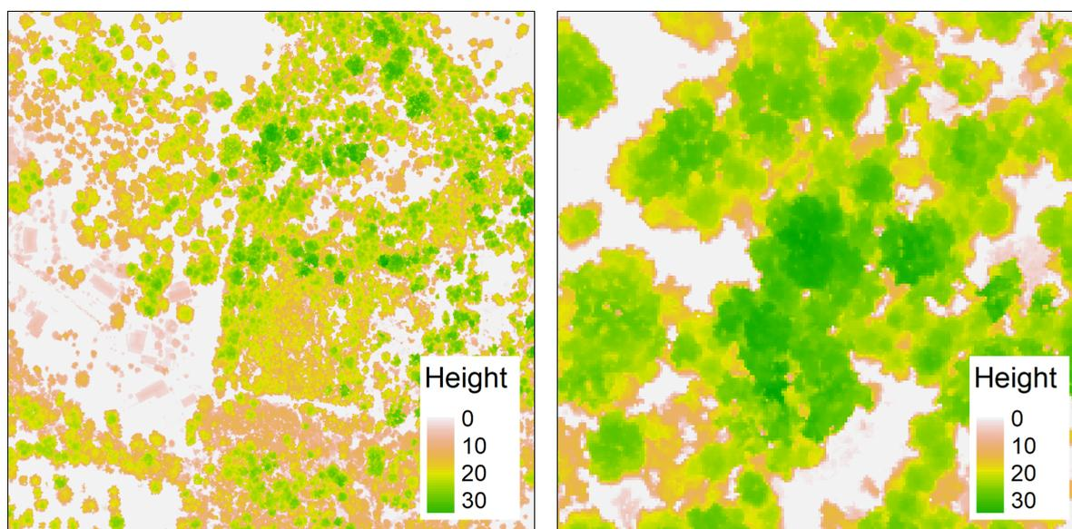
**Figure 9.** Example of a 1 m CHM derived from airborne lidar. The second image is a 'zoomed in' area of the first.
