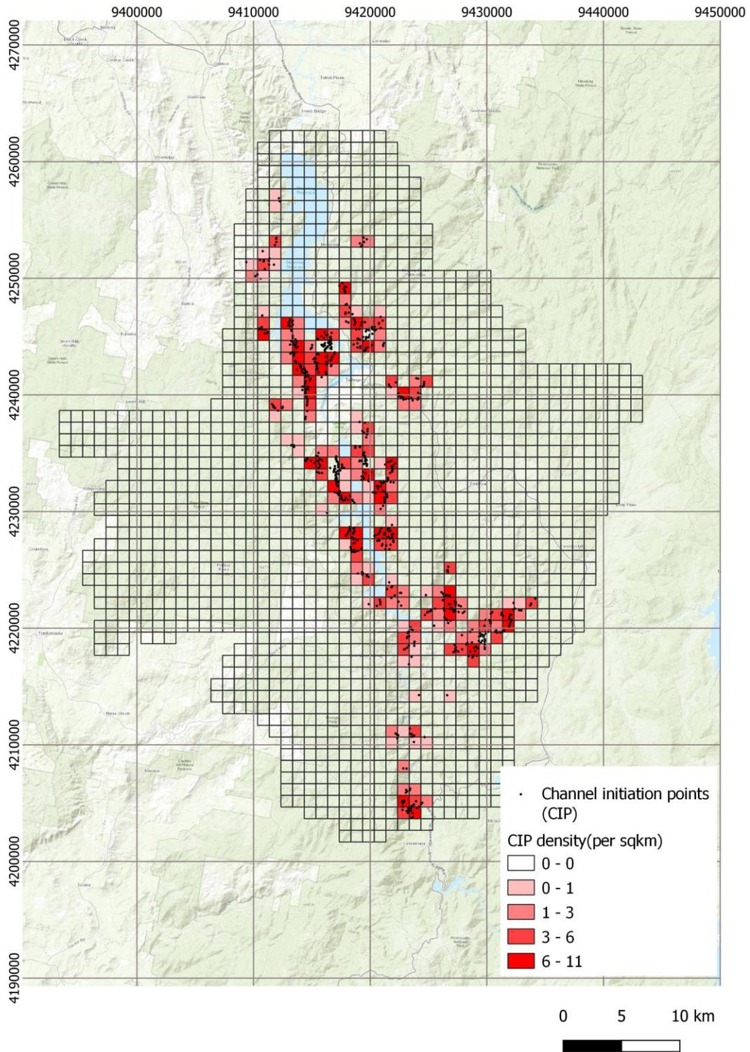
Figure 4-1. Distribution of channel initiation points (CIP) in the Tumut study area. The red color gradient is the number of CIPs per km<sup>2</sup>. Black dots are individual CIPs.
