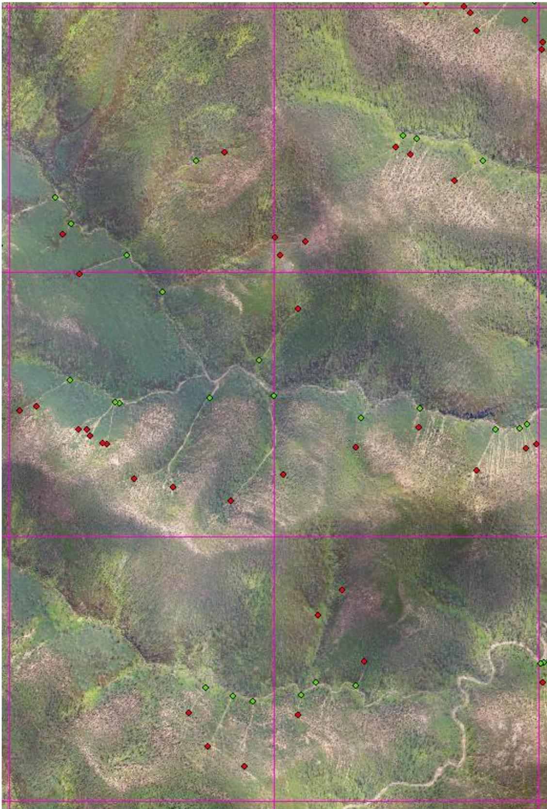
Figure 3-6. Debris flow fans (green) and channel initiation points (red) within 1km<sup>2</sup> grids.
