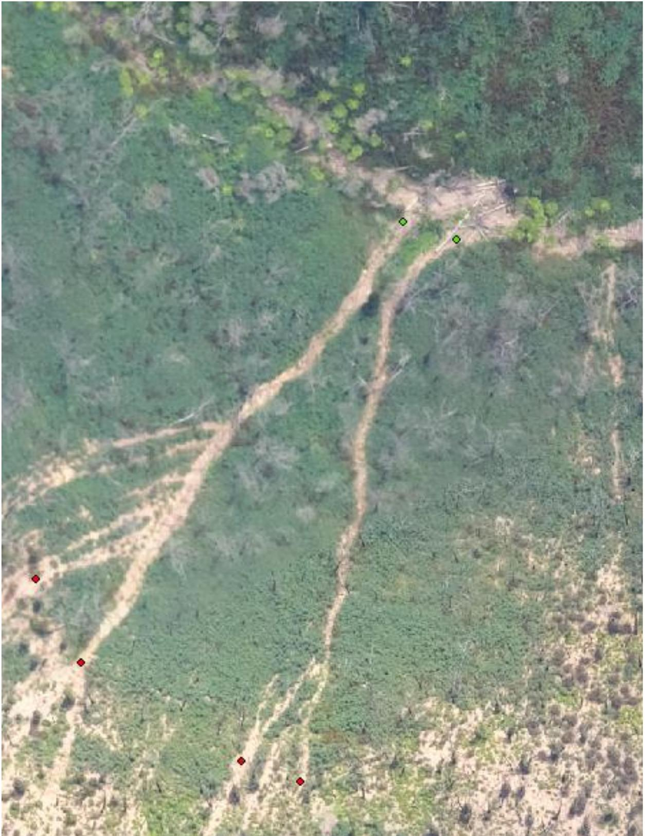
Figure 3-5. Mapping of debris flow fans (green markers) and channel initiation points (red markers).
