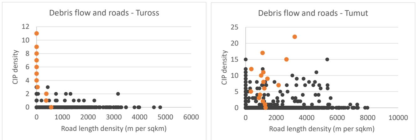
Figure 4-5. Association between road length density in each grid and the CIP density in the Tuross (left) and Tumut (right) study areas. Black markers are data pairs from each grid. The orange markers are the averages of road length density for each level of CIP density.
